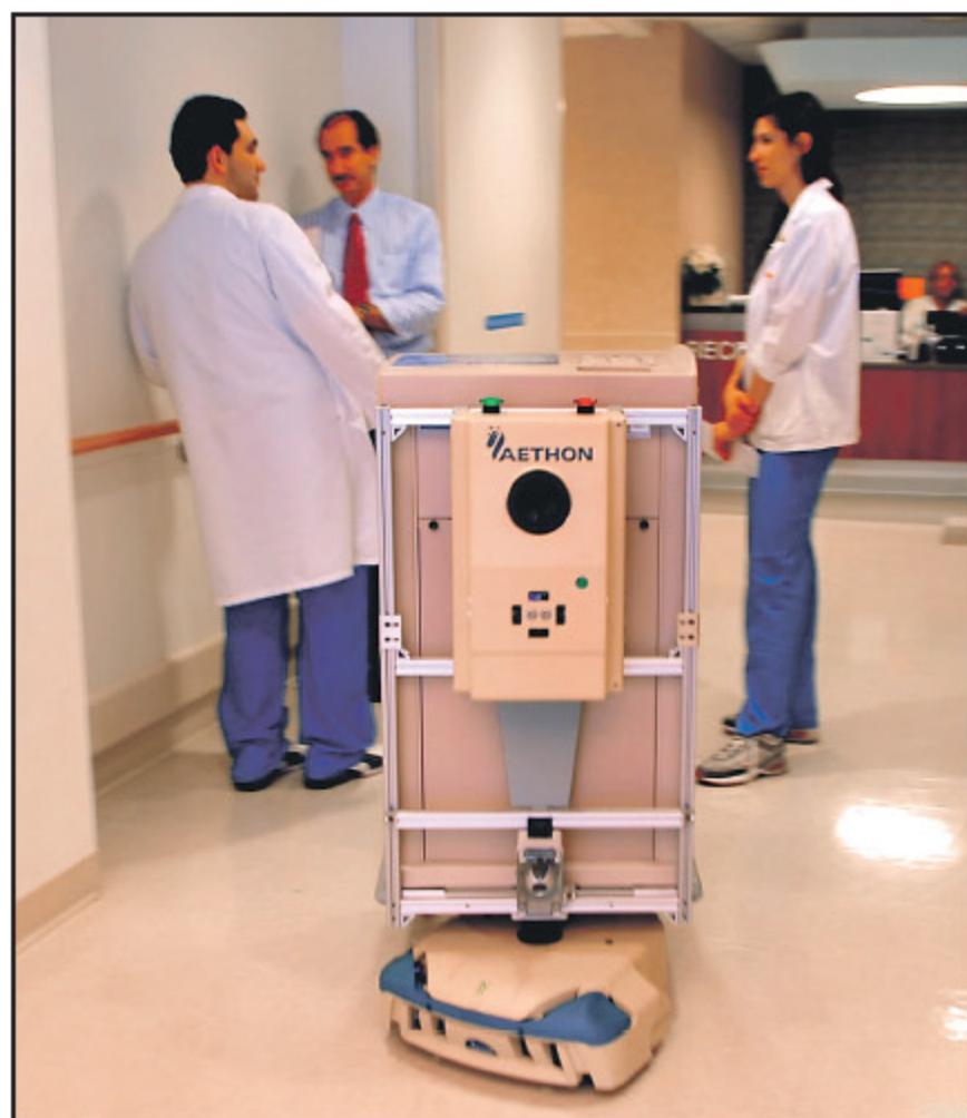
Harriet the robot delivers medication in locked compartments to departments in the hospital, even traveling on elevators without human aid.
